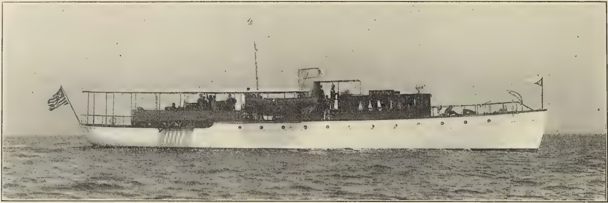
THE STEEL TWIN SCREW MOTOR YACHT CRISTINA, DESIGNED BY HENRY J. GIELOW. (Photograph, N. L. Stebbins, Boston.)
